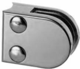
KLH10R-50.8 50.8mm D Shaped Glass Clamp 10mm Glass (Rubbers Also Available for 6, 8, 11.52, & 12mm) 304 Satin / 316 Satin / 316 Mirror
