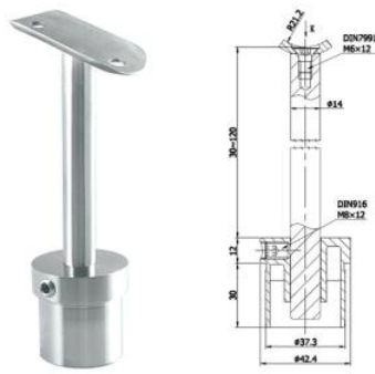
HH1005-42.4-ADJ Adjustable Bung, Stem, & Saddle 316 Grade Satin
